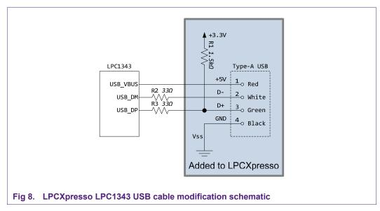
Note: Rather than building a cable or wiring a USB Type-A connector, you could take an existing A-B USB cable and cut the B connector off of it. Then the A side of the cable could be stripped and soldered onto the LPCXpresso board.
