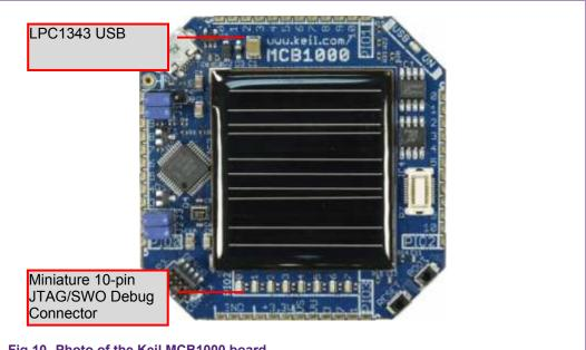
Fig 10. Photo of the Keil MCB1000 board
