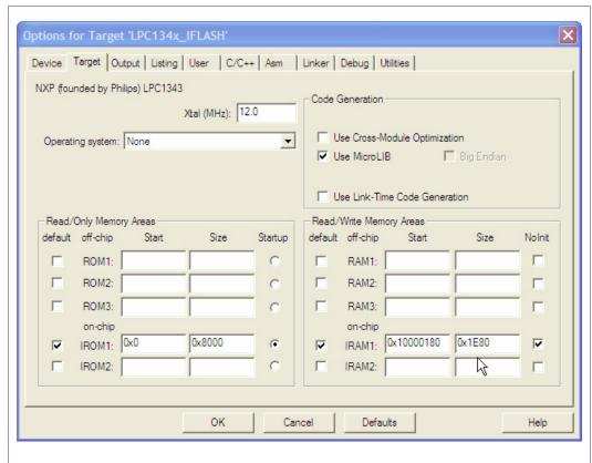
Fig 4. Keil µVision4 RealView MDK-ARM target options linker script settings
