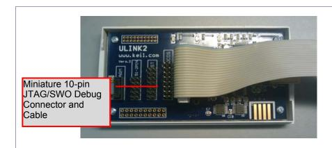
Fig 11. Photo of the Keil ULINK 2 JTAG/SWO debug interface, disassembled
